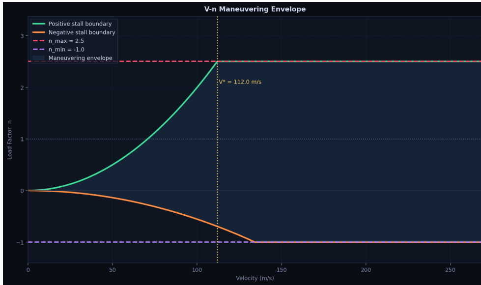
Figure 6 — V-n maneuvering envelope. Corner speed V^* = 112 \text{ m/s} (218 kt). Structural limits: n_{max} = +2.5 , n_{min} = -1.0 . The shaded region is the safe operating envelope.
